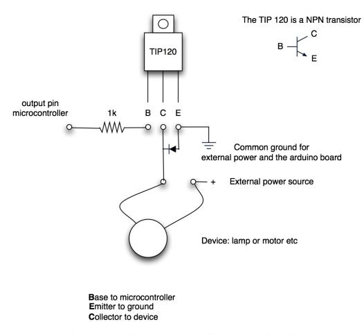
Diode from E to C when connected to inductive load like a DC motor
