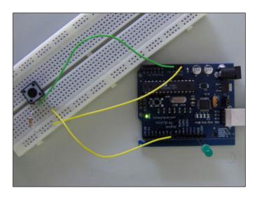
Example circuit using a push button switch: <u>http://www.arduino.cc/en/Tutorial/Button</u>
