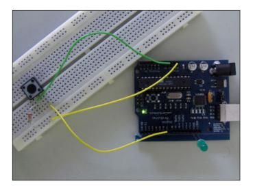
Example circuit using a push button switch: <a href="http://www.arduino.cc/en/Tutorial/Button">http://www.arduino.cc/en/Tutorial/Button</a>
