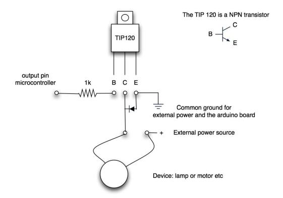
Base to microcontroller Emitter to ground Collector to device
