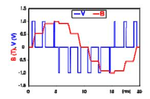
*PWM modulates the duty cycle of a square wave to control the amount of power sent out to a load.* On the Diecimila the output signal is at approximately 490 Hz.
